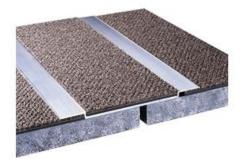
Nystrom's Double Wing Flooring Infill System is designed to cover thermal expansion joint openings. Constructed of aluminum and designed to integrate with carpet, tile and VCT flooring, this system provides a minimal 1-1/2 inch sight line.
