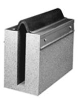
Nystrom's Roof Bellows System is an effective, flexible joint closure for a wide variety of standard and special applications. The ECF cover is 60-mil thick, reinforced EPDM bellows widely used in roof to roof and roof to wall curb applications.
