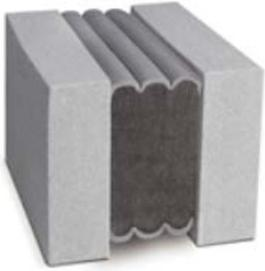
Fire-retardant floor and deck foam. Nystrom's Fire-Rated Deck Compression Seal is a silicone bellow system designed with a 2 or 3-hour fire-retardant saturated foam. It is watertight, fire-rated, and has a dual sided primary seal for both new and retrofit structural expansion joints in parking deck applications.
