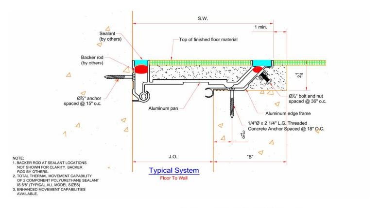
Note: Exposed Aluminum Surfaces Mill Finish (standard).
