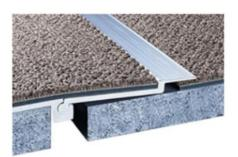
The Single Wing Hinged Flooring Infill System is designed with a hinged cover to accommodate horizontal and vertical thermal movement. This surface mounted system is designed to integrate with carpet and VCT flooring and provides a minimal sight line.
