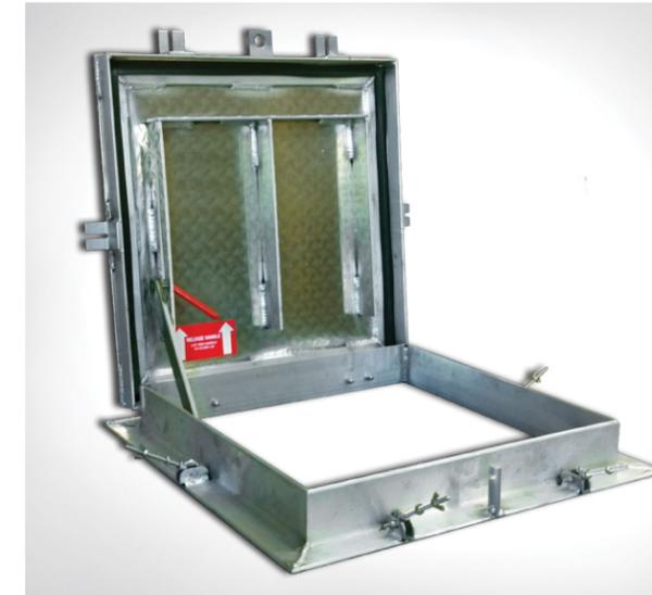
Nystrom's Water Tight Well Hatch is designed for water-tightness up to 10 foot water column and 625psf load capacity. With waterproof gaskets and pressure locks, this hatch design is ideal for wells and areas prone to flooding.
