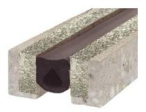
Rubber foam for stairwells and elevator shafts. The Perimeter Deck Compression Seal is constructed of flexible, closed cell neoprene expanded rubber foam seal that is adhered in place with epoxy adhesive.
