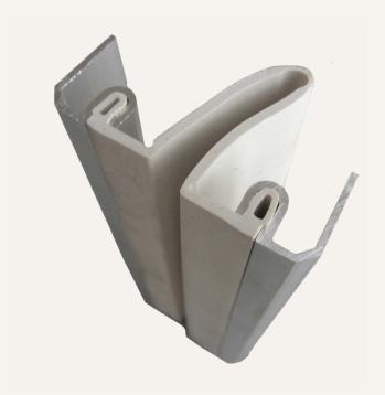
Nystrom's Seismic Elastomeric Ceiling System uses an aluminum channel attached to the grid system above the sight line. The finished Santoprene seal comes in four colors to match your surrounding substrate and finish material. This system accommodates seismic movement.
