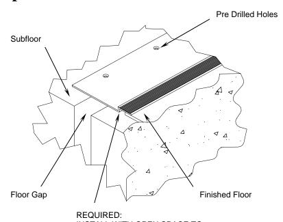
INSTALL WITH OPEN SPACE TO ALLOW FOR FLOOR MOVEMENT
