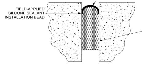
WATER-BASED, ACRYLIC-INFUSED EXPANDING FOAM ANCHORING SYSTEM
