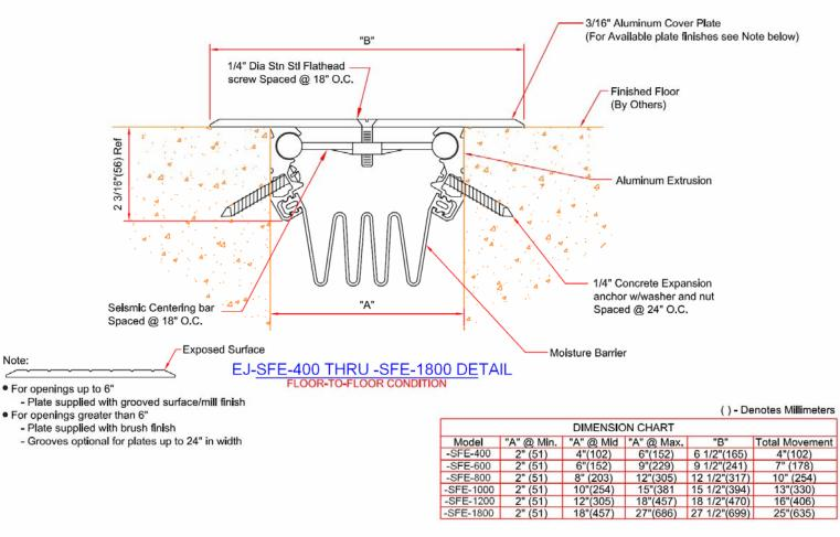
Note: Minimum And Maximum Values Are After Movement Occurs. Mid Point Value Is The Recommended Size Of Opening At Installation.
