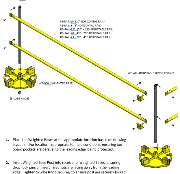
3. Attach appropriate length Horizontal Rails to Weighted Base Post by either sliding rails on to drop-lock pins or fastening in to insert rivet nuts with bolts provided. When attaching horizontal rails using bolts and insert nuts, tighten bolts to recommended torque of 70 inch pounds for clean and dry bolts.
