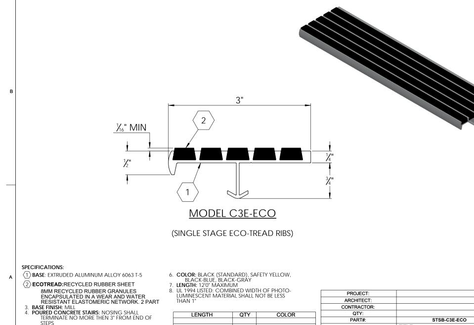
5. CONCRETE FILLED STEEL PAN STAIRS: NOSING SHALL BE FULL LENGTH OF STEPS, LESS 1/8" CLEARANCE
