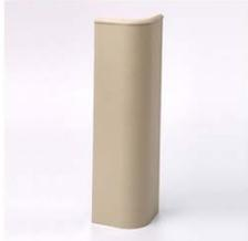
Vinyl Door Guards are designed with a 1-1/4" radius cover that is mounted over a continuous aluminum cover. The top and bottom caps "lock" the profile cover in place while the retainer can be modified to fit most door frame styles.
