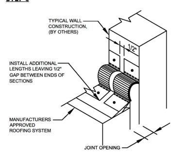
REPEAT STEPS 1 THRU 5 FOR REMAINING SECTIONS, BEING SURE TO PROVIDE ½" GAP BETWEEN ENDS OF SECTIONS.
