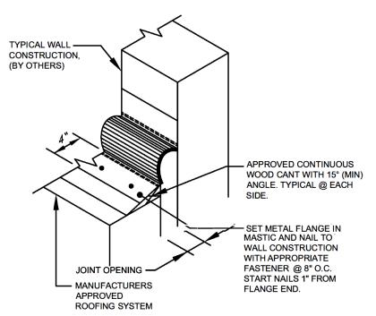
SET FLANGE IN MEMBRANE COMPATIBLE MASTIC AND NAIL TO WOOD CANT W/ (1) 1¾" ROOF NAI L @ 4" O.C. START NAILS 1" FROM FLANGE END.
