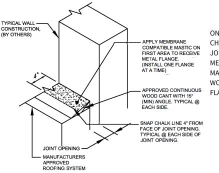
ON THE ROOF SIDE, SNAP A CHALK LINE 4" FROM FACE OF JOINT OPENINGS. APPLY MEMBRANE COMPATIBLE MASTIC ON 4" WIDE AREA OVER WOOD CANT TO RECEIVE METAL FLANGE.
