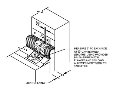
MEASURE 3" TO EACH SIDE OF ½" GAP BETWEEN LENGTHS.
