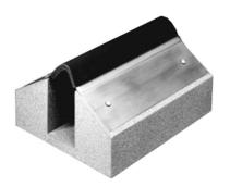
Nystrom's Roof Bellows System is an effective, flexible joint closure for a wide variety of standard and special applications. The EEJ cover is 60-mil thick, reinforced EPDM bellows widely used in roof to roof and roof to wall cant applications.
