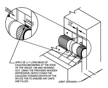
APPLY 1/4" x 1" LONG BEAD OF CAULKING BEGINNING AT THE EDGE OF THE SPLICE TAB AND WORKING OUT. USING THE PROVIDED WOODEN DEPRESSOR, GENTLY DRAG THE CAULKING TOWARD CENTER OF THE SPLICE TAB TO ENSURE ANY GAPS ARE FILLED. TYPICAL @ FOUR LOCATION PER SPLICE TAB AND TYPICAL @ EACH SPLICED LOCATION.
