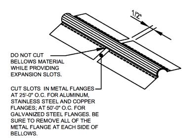
FOR ROLLED EEJ PRODUCTS; CUT SLOTS IN METAL FLANGES TO ALLOW EXPANSION. CUT SLOTS AT 25'-0" ON-CENTER FOR ALUMINUM, STAINLESS STEEL AND COPPER FLANGES; AT 50'-0" ON-CENTER FOR GALVANIZED FLANGES. PROVIDE FULL SPLICE AT EACH OF THESE LOCATIONS AS DESCRIBED IN SPLICING INSTALLATION INSTRUCTIONS BELOW.
