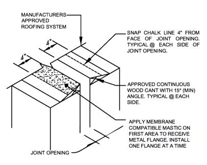
SNAP CHALK LINE 4" FROM FACE OF JOINT OPENINGS, TYPICAL @ EACH SIDE OF JOINT OPENING. APPLY MEMBRANE COMPATIBLE MASTIC ON 4" WIDE AREA OVER WOOD CANT TO RECEIVE METAL FLANGE. INSTALL ONE FLANGE AT A TIME.
