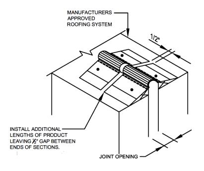
REPEAT STEPS 1 THRU 3 FOR REMAINING SECTIONS OF EEJ BEING SURE TO PROVIDE ½" GAP BETWEEN ENDS OF SECTIONS. PROVIDE FULL SPLICE AT EACH OF THESE LOCATIONS AS DESCRIBED IN THE SPLICING INSTALLATION INSTRUCTIONS BELOW.
