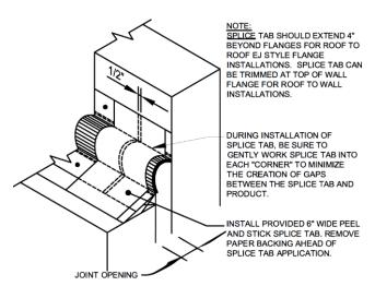
INSTALL PROVIDED 6" WIDE PEEL AND STICK SPLICE TAB. REMOVE PAPER BACKING AHEAD OF SPLICE TAB APPLICATION BEING SURE NOT TO STRETCH THE SPLICE TAB AND WORKING IT INTO EACH CREVICE. SPLICE TAB MUST EXTEND AN
