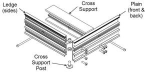
If there are cross supports, insert them between the plain side frame sections and attach them with the remaining screws. When the frame is completely assembled, finish tightening all screws. Install the support posts for the cross supports on the bottom of the supports as indicated in the shop drawings. Adjust support post heights as necessary.
