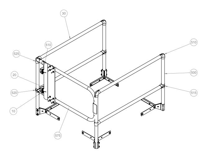
ITEM NO. PART NUMBER DESCRIPTION QUANTITY 27496-4.00-Y RAIL, 1-1/4" X 4.00L, 10 2 20 27496-18.00-Y RAIL, 1-1/4" X 18.00L, 1 30 27496-48.50-Y RAIL, 1-1/4" X 48.50L, 4 PKG, CORNER POST, ALUM 500 27180-A-Y 4 510 27185 FTG, ELBOW, 5 27188 FTG, TEE, 3 515 FTG, CROSS ELBOW, 520 27186 1 FTG, DBL TEE, 525 27231 1 GATE, 30, SRCA-GATE-30 1 575
