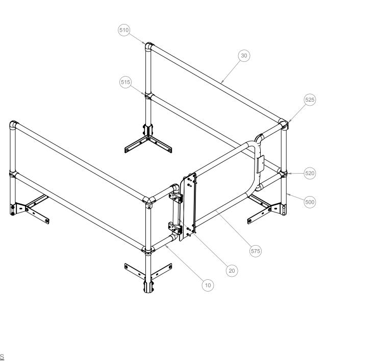
ITEM NO. PART NUMBER QTY. DESCRIPTION 27496-10.50-Y 4 RAIL, 1-1/4" X 10.50L, 27496-18.00-Y 2 RAIL, 1-1/4" X 18.00L, 20 27496-60.50-Y 4 RAIL, 1-1/4" X 60.50L, 30 500 27180-A-Y 4 PKG, CORNER POST, ZPS, 27185 FTG, ELBOW, 510 6 515 27188 2 FTG, TEE, FTG, CROSS ELBOW, 520 27186 2 FTG, DBL TEE, 575 SRCAY-GATE-30 1 GATE, 30,
