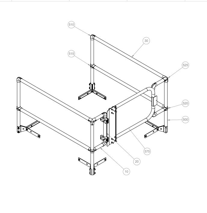
ITEM NO. PART NUMBER **DESCRIPTION** QTY. 27496-8.00-Y RAIL, 1-1/4" X 8.00L 4 27496-18.00-Y RAIL, 1-1/4" X 18.00L, 2 20 30 27496-55.75-Y RAIL, 1-1/4" X 55.75L, 4 PKG, CORNER POST, ZPS, 500 27180-A-Y 4 27185 510 FTG, ELBOW, 6 2 515 27188 FTG, TEE, FTG, CROSS ELBOW, 520 27186 2 FTG, DBL TEE, 2 575 SRCAY-GATE-30 GATE, 30, ALUMINUM, YELLOW
