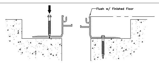
Secure extrusions to slab by following manufacturers recommendations for proper anchor installation.
