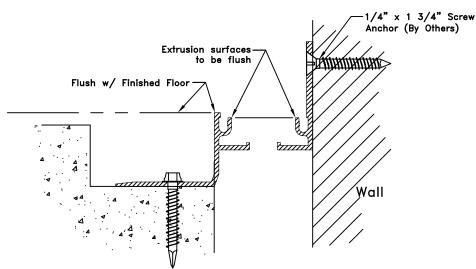
Secure extrusions to slab by following manufacturers recommendations for proper anchor installation. Use 2" section of seal on both ends of extrusion as guage to ensure proper separation. Along corner condition use the proper anchor (supplied by others) to mount wall Extrusion to wall. Note: Wall mount estrusion not pre—drilled by manufacturer.
