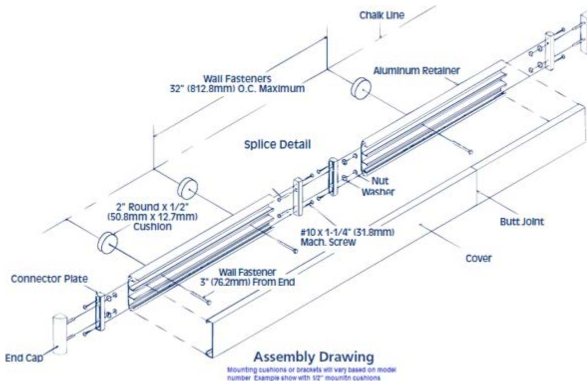
**Installation Dimensions for CRVS4C, CRVS4C-C125 (1/8" mounting cushion), CRVS4C-C05 (1/2" mounting cushion), CRVE4C-B15 (1 1/2" mounting bracket) and CRVE4C-B2 (2" mounting bracket).**
